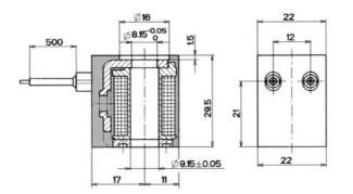
22 mm coils for valves type MH, MNH and MOH; the 22 mm valves programm.
